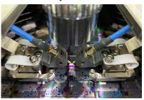
RF LTM probe arms, equipped with SmartCarrier™
