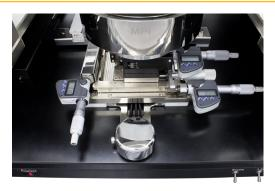
MPI offers the worldwide unique and most accurate contact / over-travel control with 1  $\mu m$  accuracy for easy measurement reproducibility and accuracy.
