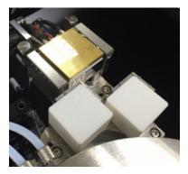
MPI auxiliary chucks made by ceramic
