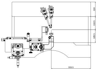
Probe Platen design for DC, RF and THz MicroPositioners
