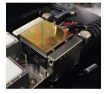
Thermal chuck system for testing single ICs
