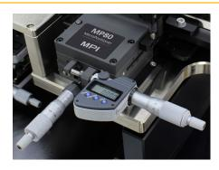
The optional MP80-DX MicroPositioner with the integrated digital micrometer enables outstanding simplicity for the multiline TRL.
