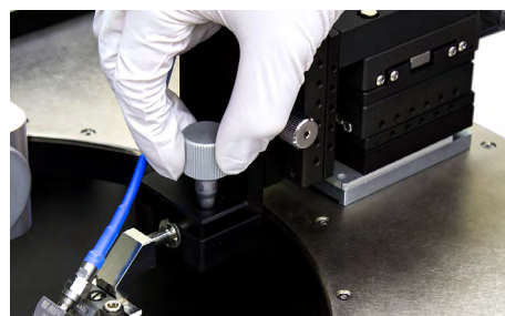
Figure 4. Planarization of TITAN™ Probes.
