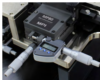
The MP80-DX MicroPositioner with the digital micrometer on the X axes.
